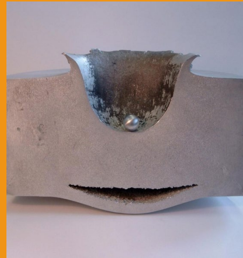
Impact of a small piece of space debris on a typical unshielded aluminum space craft skin (0.5mm debris)
